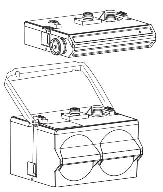
Figure 2-6 Assembling a basic portable system
